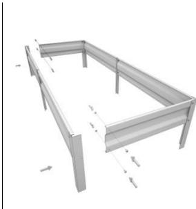
5. Next to the resulting structure at the junction of the side panels fasten the screed with screws (as in Fig. 13)
