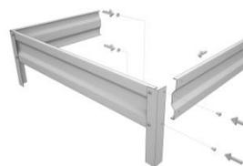
3. Then connect the remaining side panel with the resulting structure (as in Fig. 6). The garden-bed is ready (as in Fig. 7), set in the ground.
