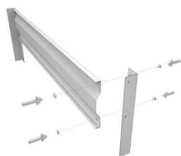
2. Next, screw the face end panel to the side panel (as in Fig. 4), and then screw the second face end panel to the same side panel (as in Fig. 5)
