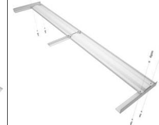
3. Next, screw the face end panel to the side panel, and then screw the second face end panel to the same side panel (as in Fig. 11).
